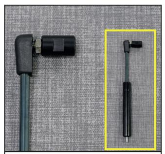
**1.1** Attach the **Gas Spring Boss** to the **Gas Spring** nipple. Tighten securely using the 8mm and 10mm Spanners.
