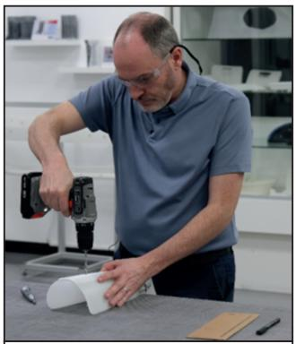
**2.11** Use the Hand Drill and 5.5mm Drill Bit to drill the x3 marked hole positions.
