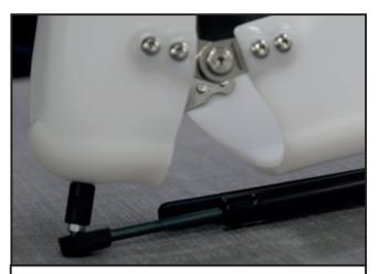
**3.4** Re-attach the **Gas Spring** to the Gas Spring Nipple. It is advised to place the CCD Lever Kit onto a hard surface (table or workbench) and press the **Gas Spring Boss** and Nipple which is attached to the CCD Shell into the **Gas Spring**.
