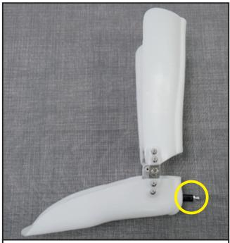
**3.2** Attach the **Gas Spring Boss** to the Heel. Use the 3mm Allen Key and 10mm spanner to tighten securely. Use one of the M5 Counter Sinks Screws to fix.
