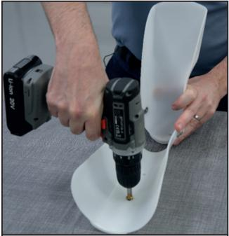
**2.12** Use the Counter Sink Bit and Hand Drill to remove any burrs from both sides of the drilled holes. Apply a 3mm Countersink to the inside face of the CCD Shell to all 3 holes.
