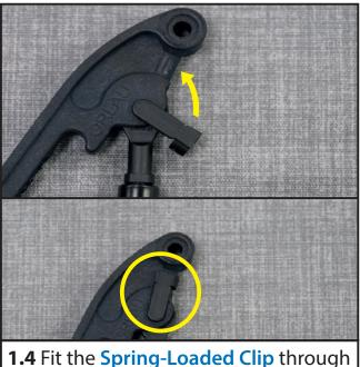
**1.4** Fit the **Spring-Loaded Clip** through the **Lever** and **Rod End**, rotate anticlockwise and engage the **Spring-Loaded Clip** onto the **Lever**. NOTE: Do not fit the **Spring-Loaded Clip** to the **Rod End**. It must be fitted to the **Lever**.
