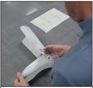
**2.6** After marking the CCD Shell check the angle set in 2.1 has been unaltered using the Goniometer.
