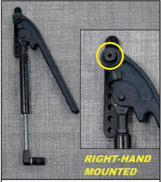
**1.5** Decide which side the Lever is to be placed on the CCD Shell and rotate accordingly. Fit the Lever to the Bracket with the Shoulder Screw. Fit to the 3rd hole from the top of the Bracket with the 3mm Allen Key.
