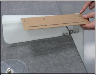
**2.7** Place the CCD on a work surface with the foot section over hanging the edge of the working area (being careful not to move the ankle joint angle set in Step 2.1). Detach the template for marking drill hole positions from the kit box and align the bottom v-cut (marked "HEEL") with the cross-hair previously drawn on the CCD heel apex.
